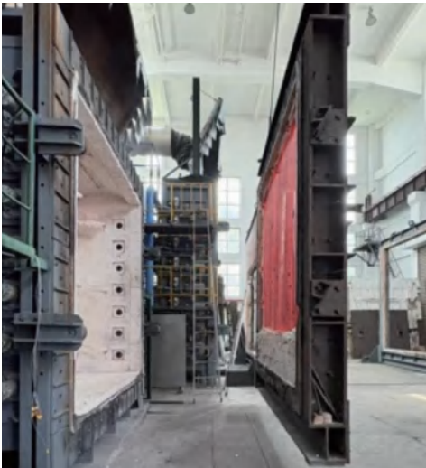
A bulkhead fire test furnace
